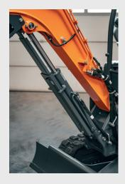
Arm, boon bucket cylinder protections engineered to withstand the challenging job site environments, ensuring longevity and durability for your equipment.
