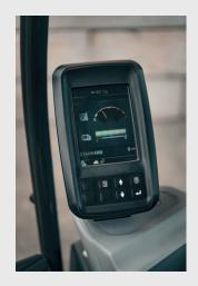
The easy-to-read, full-color, 5,7' LCD screen displays key machine data and control options.
