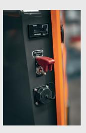
The strategically positioned emergency cut-off button provides instantaneous disruption of all machine functions, swiftly halting operations in critical situations.
